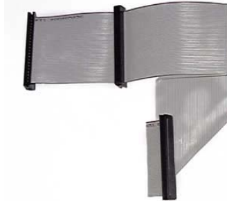
Figure 3: IDE Cable – See instructor and/or Lab tech for help hooking this up to Altera DE-1 Board
