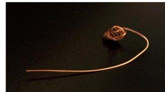
Figure 4. Mg ribbon wrapped in copper wire
