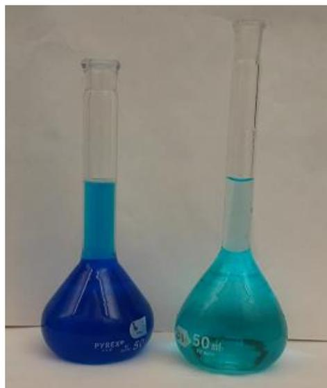
**Figure 1:** Solutions of copper(II) nitrate; the solution on the left is 1.0 M and the solution on the right is 0.10 M.
