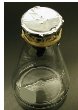
Figure 2. Flask with foil and small pin holes.
