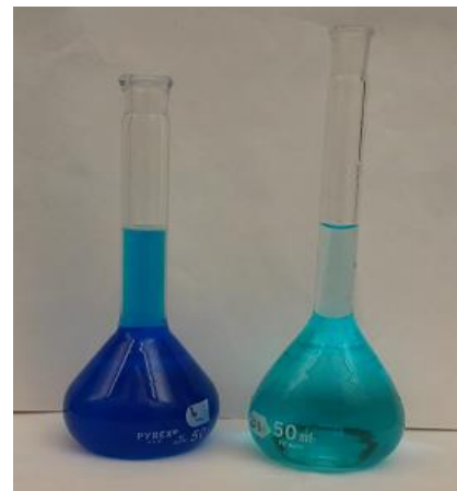
Figure 1: Solutions of copper(II) nitrate; the solution on the left is 1.0 M and the solution on the right is 0.10 M.
