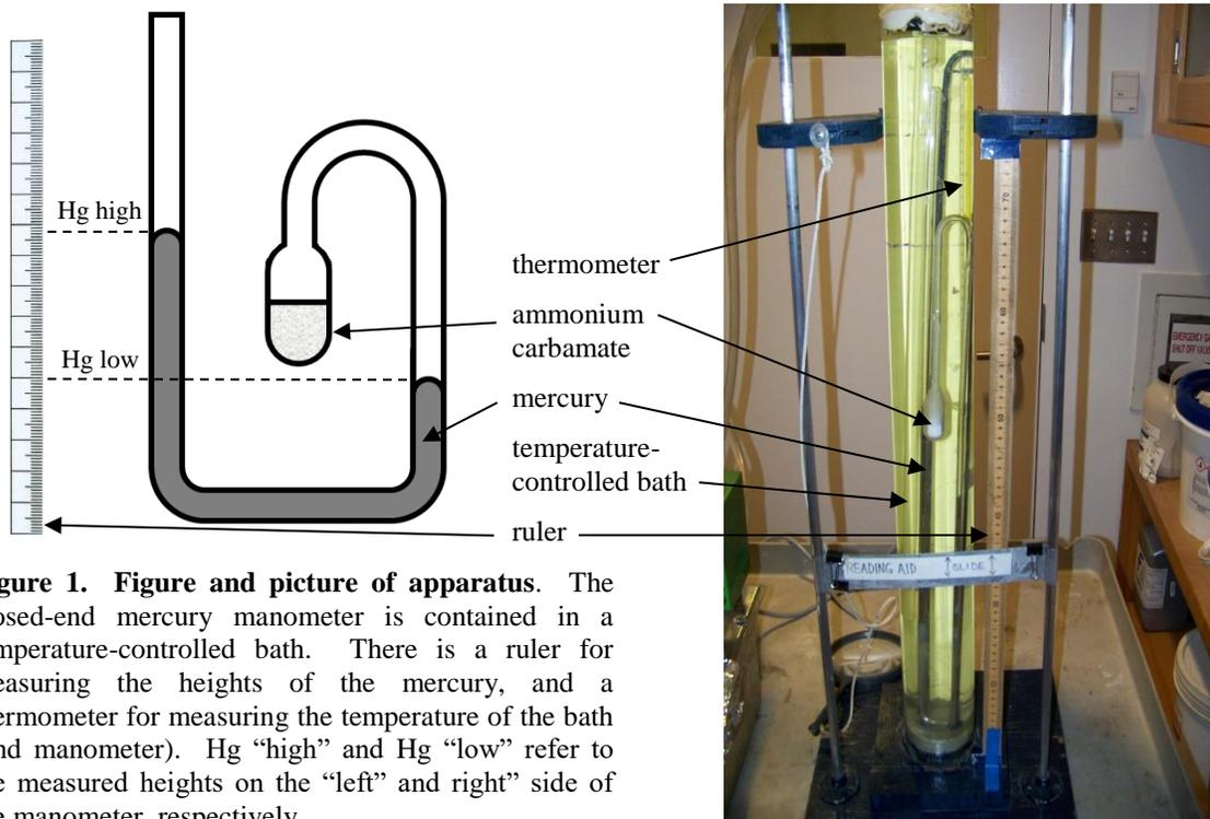
**Figure 1. Figure and picture of apparatus.** The closed-end mercury manometer is contained in a temperature-controlled bath. There is a ruler for measuring the heights of the mercury, and a thermometer for measuring the temperature of the bath (and manometer). Hg “high” and Hg “low” refer to the measured heights on the “left” and “right” side of the manometer, respectively.
