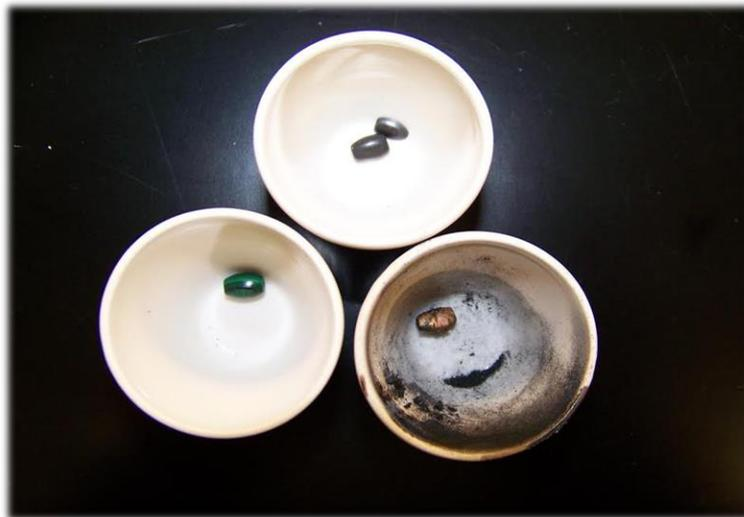
Figure 1: Malachite, Copper (II) oxide, and elemental Copper
