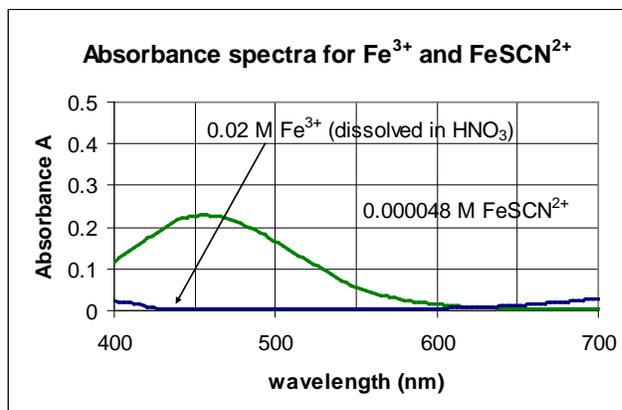
2. In Part A, step 4, you will experimentally determine the value of the molar absorptivity,  $\epsilon$ , for  $\text{FeSCN}^{2+}$  at your selected wavelength. Using the Beer-Lambert law, calculate an approximate value for  $\epsilon$  based on the spectrum of  $0.000048 \text{ M FeSCN}^{2+}$  provided above. The pathlength,  $\ell$ , for the cuvette is  $1.00 \text{ cm}$ .
