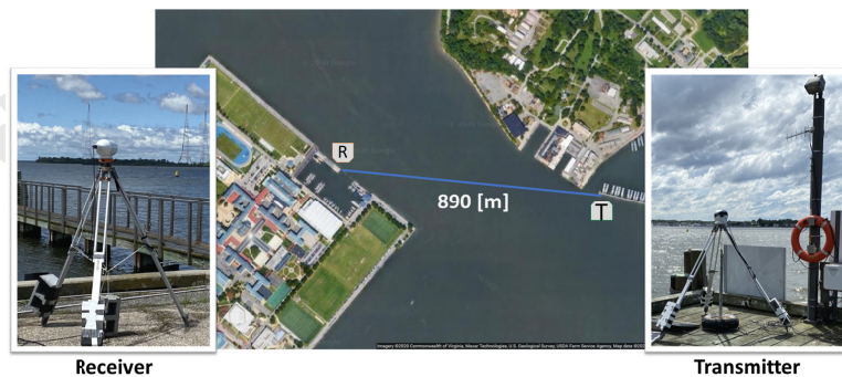
Fig. 1. Beam propagation path with receiver (left) and transmitter (right) for BLS 450 scintillometer across the Severn River in Annapolis, Maryland [18].
