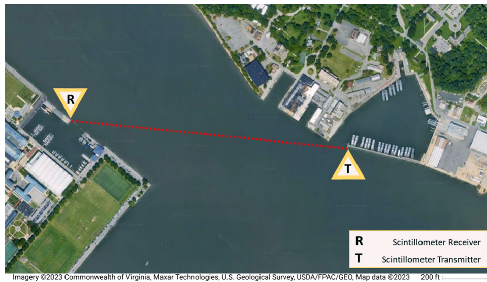
Fig. 1. Scintillometer propagation path with receiver (R) and transmitter (T) for the BLS 450 scintillometer across the Severn River in Annapolis, Maryland [16].
