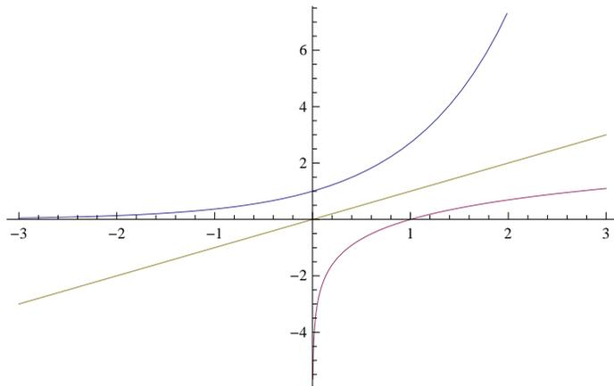
**2.3.** Plot  $\text{Exp}[x]$ ,  $\text{Log}[x]$ , and  $x$  from  $x=-3$  to  $x=3$  with the plot range of  $y$  restricted to  $[-3,3]$ .
