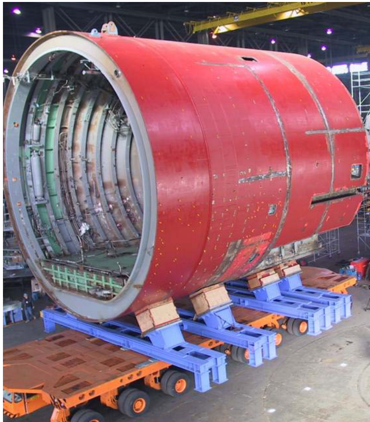
Figure 10.1 A hull section of the SSN-21 class shown during assembly. The transverse frames are shown clearly at left (the hull is a ring stiffened cylinder)
