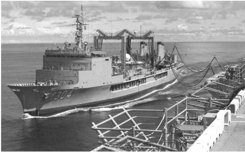
Figure 7.13 Transverse wave pattern along the hull of a replenishment ship (U.S. Navy photo)
