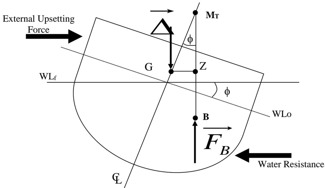
**Figure 4.1** Heeled Ship due to an External Moment
