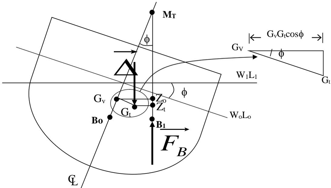
**Figure 4.7** The Cosine Correction Derivation
