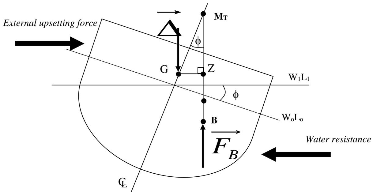
**Figure 4.13** A Ship Heeling at Small Angles
