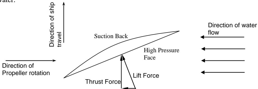
**Figure 7.20** Forces acting on a propeller blade
