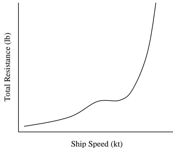
**Figure 7.5** Typical curve of total hull resistance
