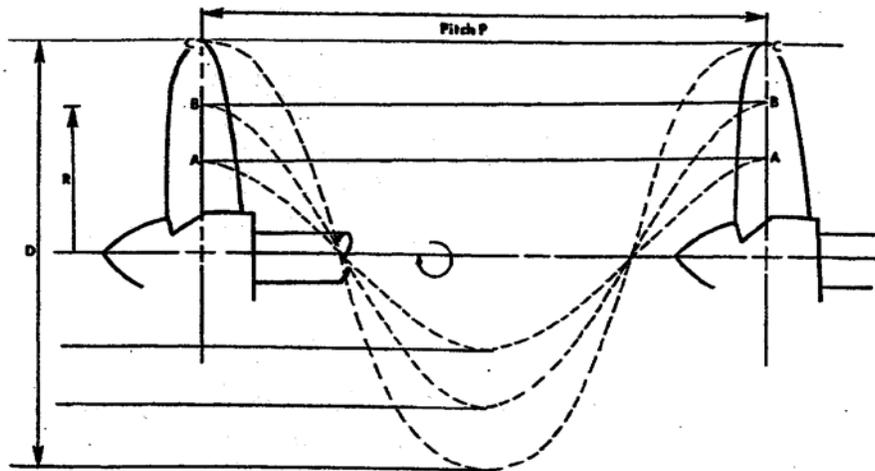
**Figure 7.19** Typical propeller operating through one revolution.
