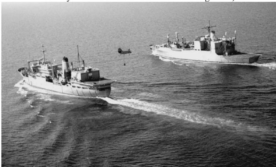
**Figure 7.12** USNS SPICA (left) conducting vertical replenishment with another ship. Note the divergent wave patterns emanating from SPICA. (U.S. Navy photo)
