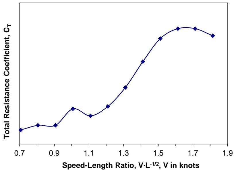
**Figure 7.16** Typical relationship between  $C_T$  and speed
