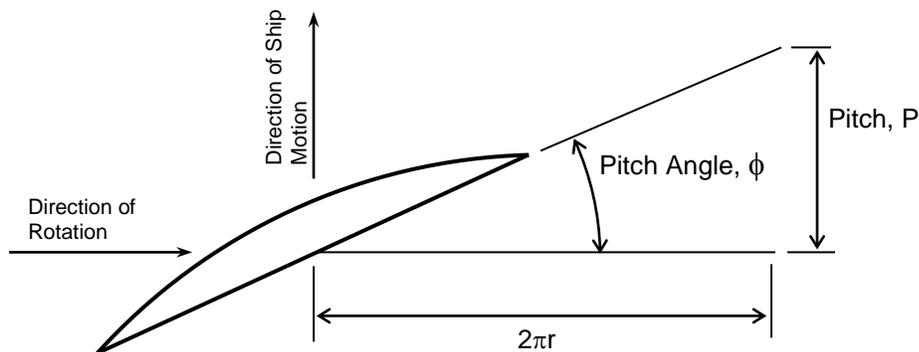
**Figure 7.18** Relationship between propeller pitch and pitch angle
