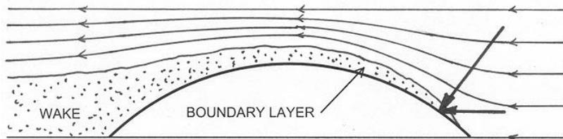
Figure 7.8 Flow around a body submerged in water
