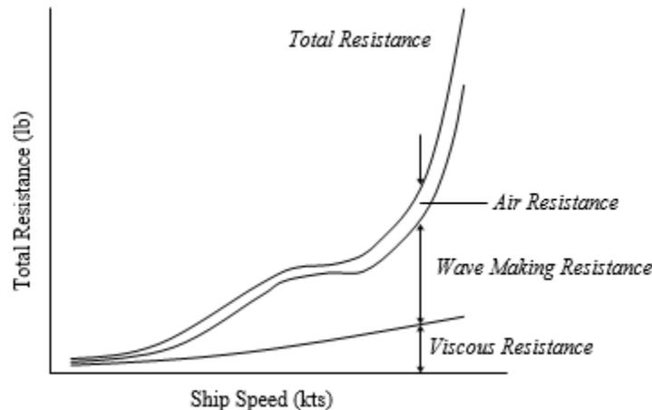
**Figure 7.6** Components of Hull Resistance
