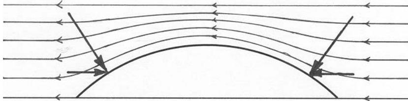
Figure 7.7 Ideal flow around a submerged body
