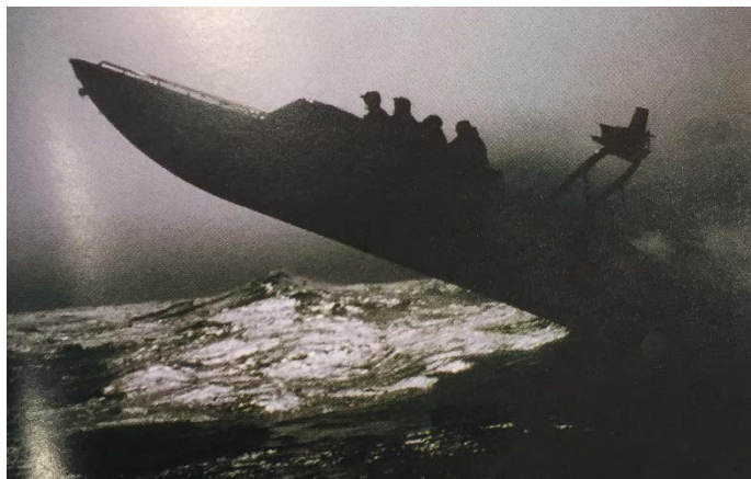
Figure 8.18 SEAL Team 6 operators experience slamming in high-speed assault craft
