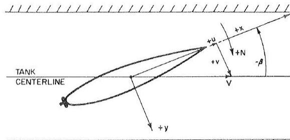
Fig. 31 Orientation of model in towing tank to determine  $Y$  and  $N$  (Abkowitz, 1964)
