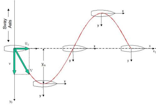
Figure 7.2: Pure Swaying Mode Test Conditions
