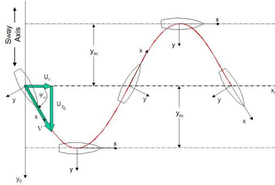
Figure 7.3: Pure Yawing Mode Test Conditions
