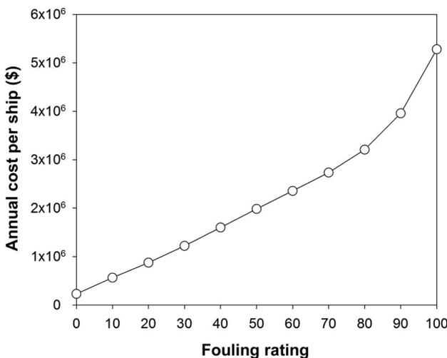
Figure 8. The annual costs (per ship) for a range of hull fouling levels (FR). The cleaning and coating costs are assumed to be the same as present practice (Case 3).
