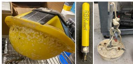
Figure 2. Left to right. SOFAR Spotter wave buoy used to collect surface wave, wind, temperature, and barometric pressure data; RBR pressure sensor used to record pressure readings at 3 meters depth; mooring made of cement base and pipe stem for RBR pressure sensor attachment.
