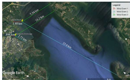
Figure 4. Fetch distances calculated for each wind event for both Annapolis Anchorage and Hackett Point using Google Earth Pro. A southeast wind and a northeast wind display a larger fetch distance at Hackett Point. In opposition, a northeast wind displays a greater fetch distance at Annapolis Anchorage.
