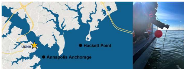
Figure 1. Locations of sensor deployment at Hackett Point and Annapolis Anchorage within the Upper Chesapeake Bay study area (left); Deployment of the RBR pressure sensor at Hackett Point (right).
