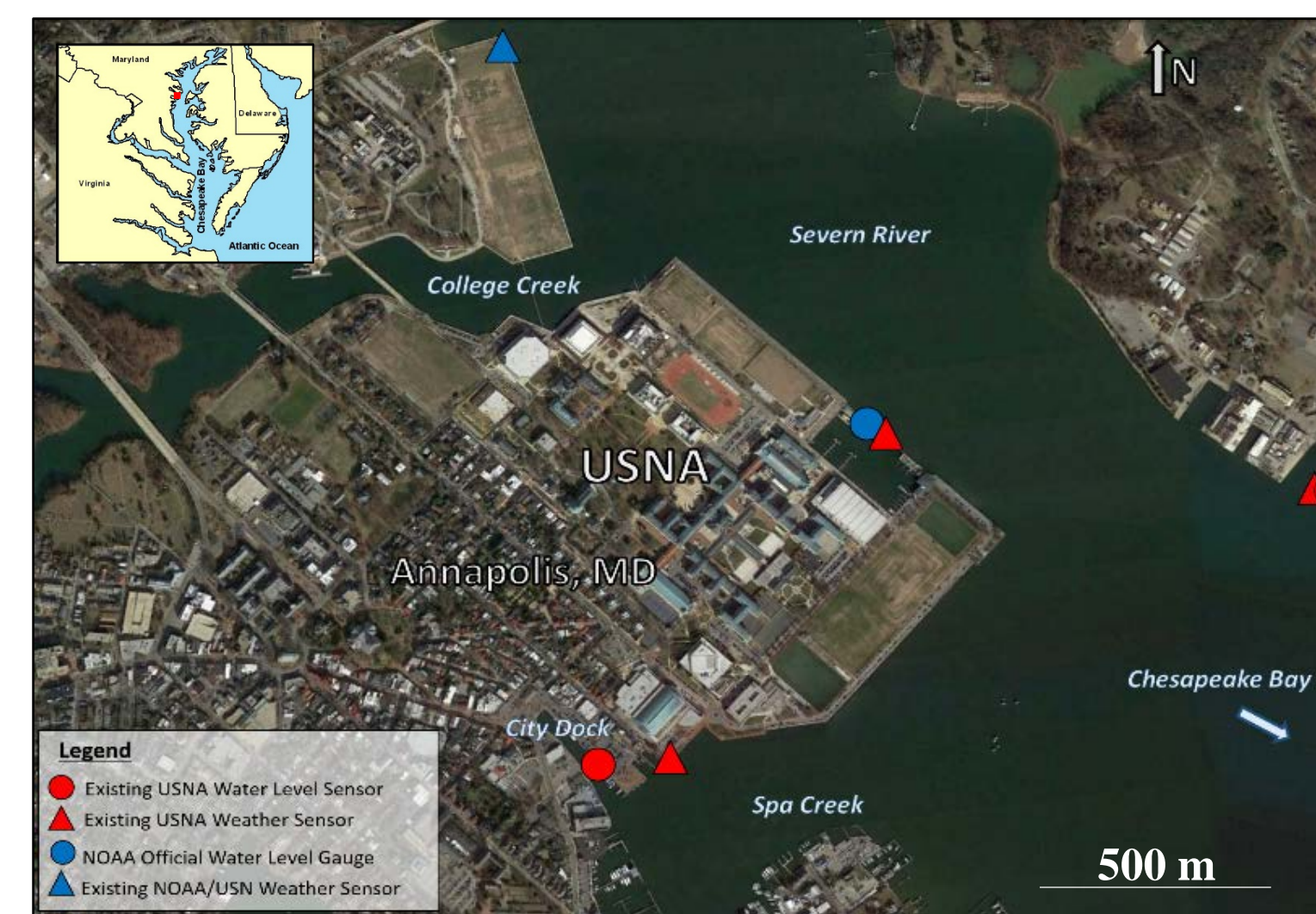
Figure 3. Map of study area in Annapolis, MD near USNA and Annapolis City Dock. Triangles mark the locations for meteorological data collection and circles mark the locations of water level and/or water pressure measurements. Blue symbols indicate NOAA data collection locations while red symbols indicate USNA Oceanography Department sensor deployments (e.g. SRWO). The RBR Solo pressure sensor was deployed at a fixed depth on a piling at the City of Annapolis Harbormaster slip in City Dock, Annapolis, MD.
