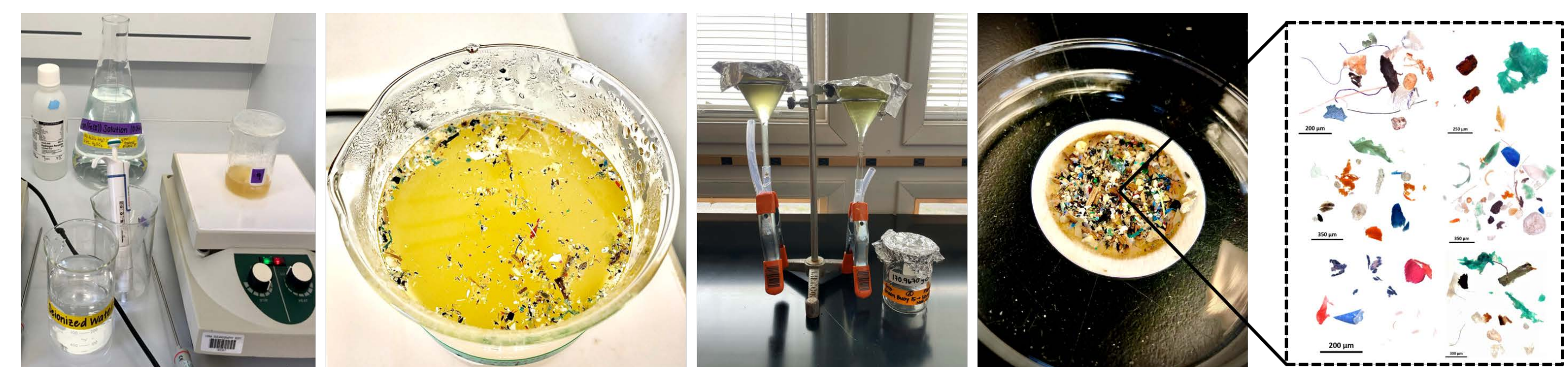
Figure 3. (Left to Right) Samples undergoing wet peroxide oxidation (WPO) – contents were treated with 20 mL aqueous 0.05M Fe(II) solution and 20 mL of 30% hydrogen peroxide that were heated to 75°C; Six grams of sodium chloride were added per 20 mL of WPO sample solution to increase density and allowed to cool; WPO and salt solution were transferred to a density separator, loosely covered with aluminum foil, and allowed to settle overnight; Floating solids from density separation were collected on a pre-weighed Whatman filter and allowed to dry and; images of microplastic and synthetic particles were collected from processed samples.
