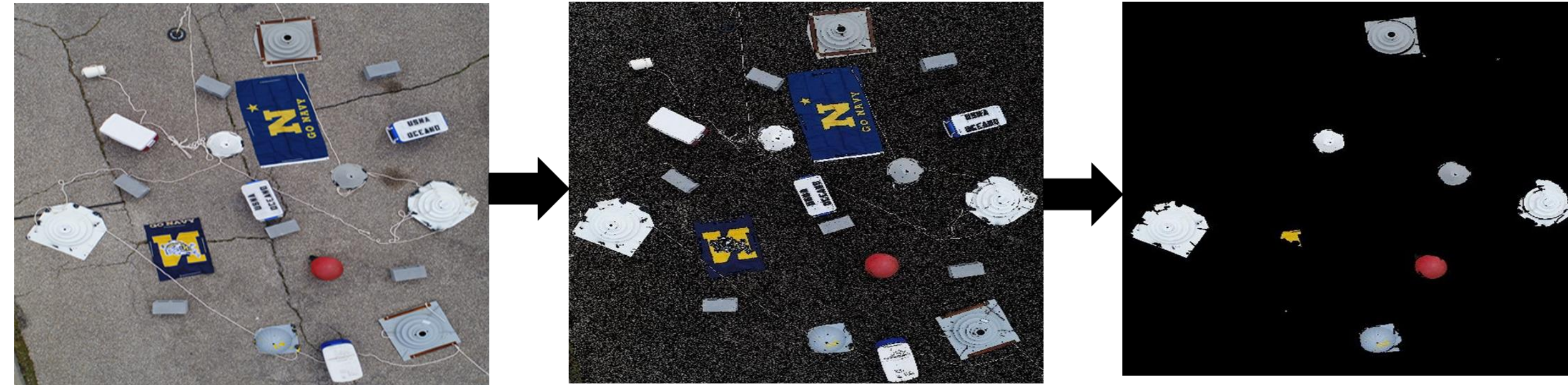
Figure 4. Series of images showing processing (left-to-right) of a control image of a land-based string of test targets taken by a DJI Phantom 4, to a RGB color segmented image, to an image showing positively identified objects that met object threshold criteria.
