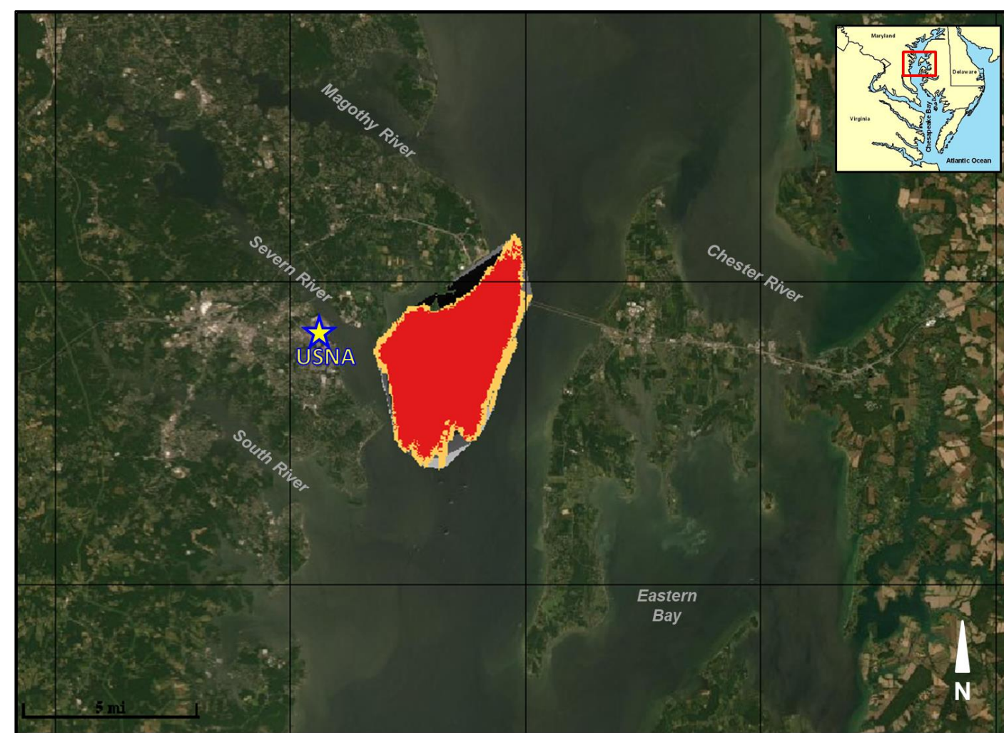
Figure 1. Results of a 30-day SHARC (v 4.0.0) simulation starting on 01 October 2019 for an instantaneous polygon release of 10,000 gallons of a conservative agent into the mesohaline Chesapeake Bay near the mouth of the Severn River near the U.S. Naval Academy (USNA). Hydrodynamic forcing was downloaded from the SHARC Tidal Harmonic Database (THDB). No meteorological forcing was included. Water column parameters such as temperature, salinity, pH were determined from the SHARC seasonal profiles database (SPDB).
