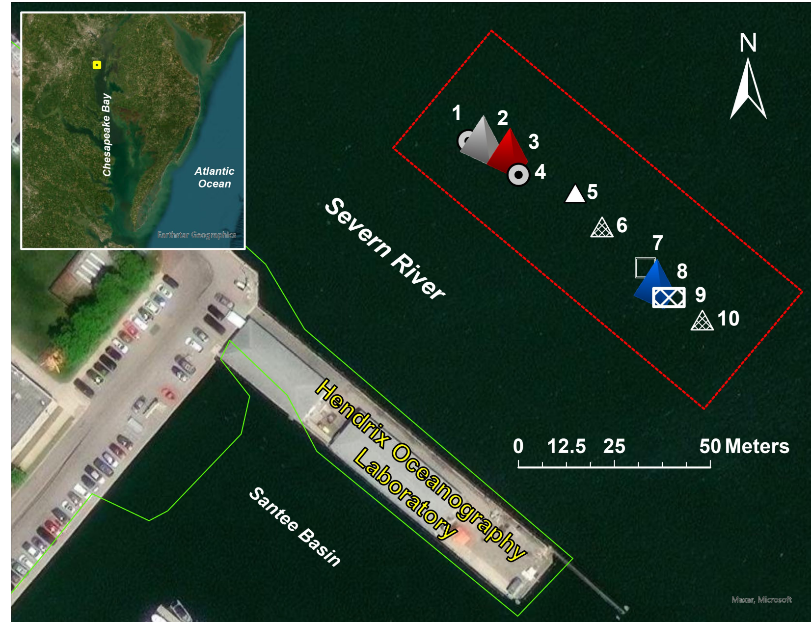
Figure 1. Map of study area at the U.S. Naval Academy (USNA) Hendrix Oceanography Lab pier, Annapolis, MD showing underwater target deployment. On 21 February 2024, 10 targets were deployed in the following order: 1 - cement control; 2 - Al-frame pyramid w/ bare Al sheet; 3 - Al-frame pyramid w/ Al sheet and Al mesh; 4 - cement control; 5 - 18" pyramid crab pot w/ silicone blanket; 6 - 18" pyramid crab pot; 7 - 36"x36" PVC frame; 8 - Al-frame pyramid w/ Al sheet and foam; 9 - 36"x24" crab pot and; 10 - 8" pyramid crab pot. The targets chosen for analysis were targets 1, 2, 3, 4, and 8. Targets were imaged during three separate surveys using a dual-frequency 455 kHz/900 kHz Klein S4900 sidescan sonar.
