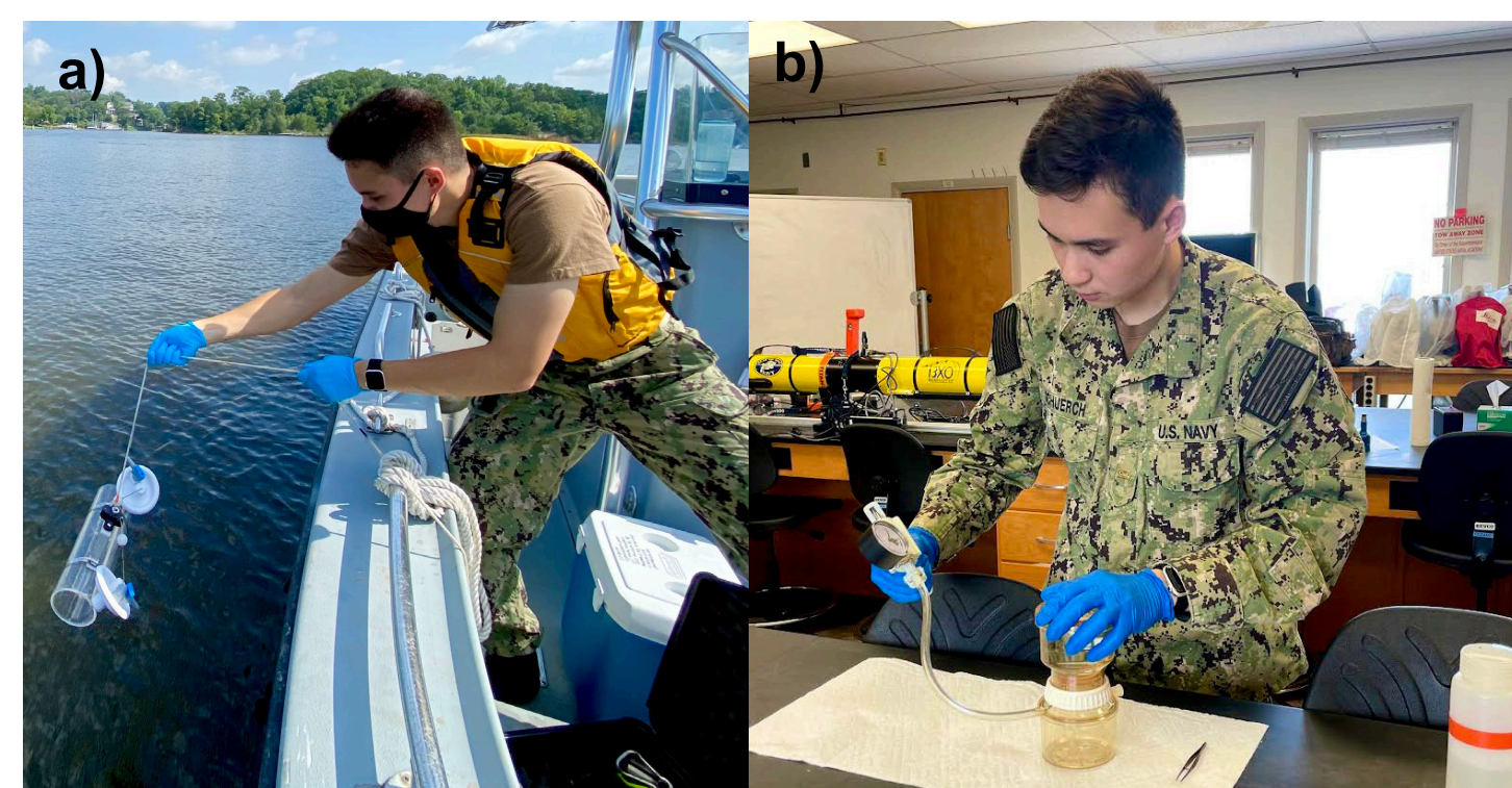
Figure 2. a) Midshipman 1/C Alex Schuerch collecting a water sample from a small boat on the Severn River using a Van Dorn bottle and b) vacuum filtering a 250 ml water sample at HOL for gravimetric analysis of TSS concentrations in the Severn River.
