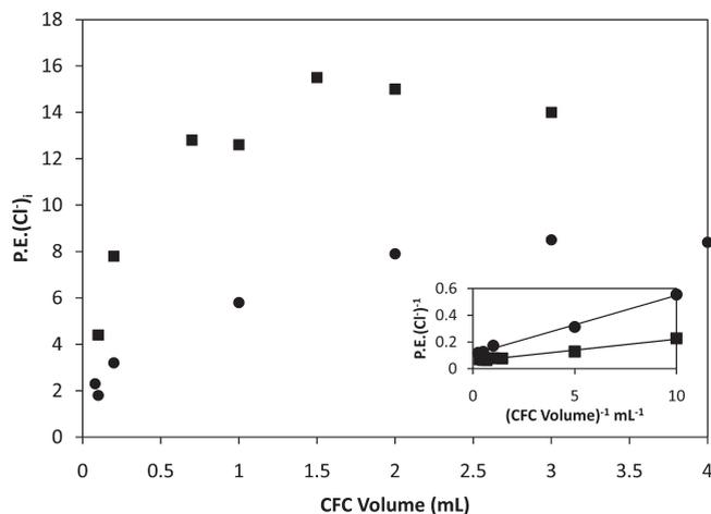
**Figure 5.**  $\text{P.E.}(\text{Cl}^-)$  vs CFC volume for Ar- (●) and air-saturated (■) suspensions containing 0.3 M  $\text{HCO}_2^-/\text{HCO}_2\text{H}$  buffer and 0.50  $\text{g L}^{-1}$  of  $\text{TiO}_2$  at pH 5.9 and irradiated with  $I_0 = 1.0 \times 10^{-6} \text{ M } h\nu \text{ s}^{-1}$ . Inset shows the same data plotted as  $\text{P.E.}(\text{Cl}^-)^{-1}$  vs  $(\text{CFC volume})^{-1}$ .
