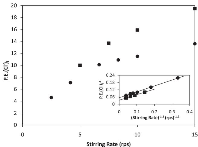
**Figure 6.** Effect of stirring rate on  $\text{P.E.}(\text{Cl}^-)_i$  for air-free (●) and air-saturated (■) suspensions containing 2.0 mL of CFC 11, 0.3 M formate/formic acid buffer, and 0.50  $\text{g L}^{-1}$  of  $\text{TiO}_2$  at pH 5.9 irradiated with  $I_0 = 1.0 \times 10^{-6} \text{ M } h\nu \text{ s}^{-1}$ . The inset illustrates the linear relationship between  $\text{P.E.}(\text{Cl}^-)_i^{-1}$  and the stirring rate raised to the  $-1.2$  power.
