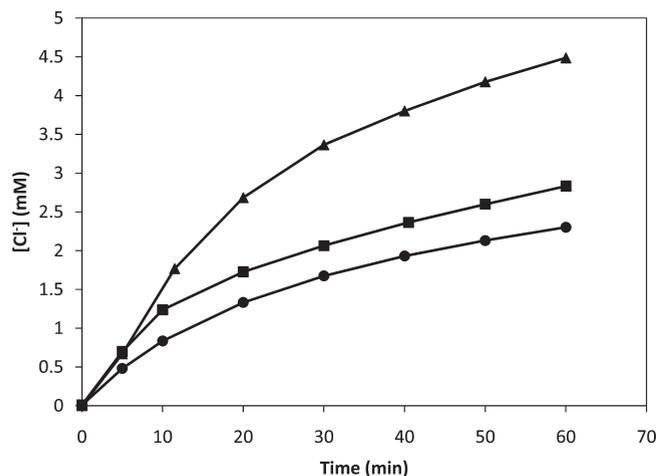
**Figure 4.** Plot of  $[\text{Cl}^-]$  vs time for Ar-saturated suspensions containing 2.0 mL (▲), 1.0 mL (■), and 70  $\mu\text{L}$  (●) of CFC 11 in the presence of 0.3 M  $\text{HCO}_2^-/\text{HCO}_2\text{H}$  buffer and 0.50  $\text{g L}^{-1}$  of  $\text{TiO}_2$  at pH 5.9 irradiated with  $1.1 \times 10^{-6} \text{ M } h\nu \text{ s}^{-1}$ .
