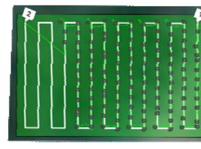
**Figure 6.** Flight path of ice rubble field on shoreline of North Star Bay, Thule, Greenland. The green line depicts the actual flight path while the white line is the intended path.
