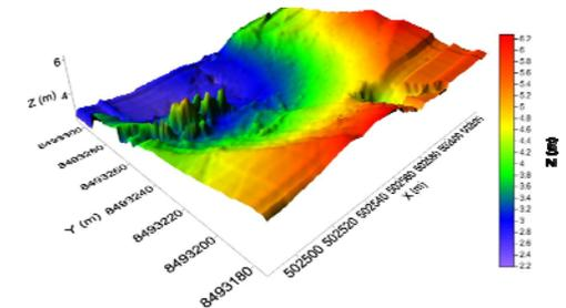
**Figure 7.** Structure from Motion (SfM) contour of ridge feature (Fig. 1B) depicted with reference to local xyz grid (Surfer v11).
