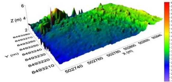
**Figure 4.** Structure from Motion (SfM) contour of rubble field (Fig. 1A) depicted with reference to local xyz grid (Surfer v11).
