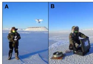
**Figure 5.** (A) DJI Phantom 4 flight and (B) laying out Ground Control Points (GCP) for survey.
