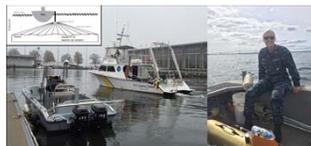
**Figure 2.** *R/V Daiber* (University of Delaware) underway at USNA with an EdgeTech 6205 Swath Bathymetry and Sidescan Sonar system, and MIDN 1/C Margo Darragh in Narragansett Bay conducting geophysical surveys with a Gavia Autonomous Underwater Vehicle (AUV).
