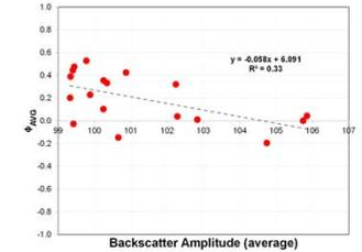
**Figure 7.** Linear relationship between  $\phi_{avg}$  and  $BS_{AMP-avg}$  values that used to estimate phi values ( $\phi_{est}$ ) for the entire survey area.
