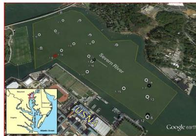
**Figure 1.** Survey area of the lower Severn River, MD (in yellow) showing the U.S. Naval Academy (USNA) and the locations of 22 sediment sampling stations chosen based on prior knowledge of the study area. The symbol for each sampling location designates a ~30 m radius around the sampling point.
