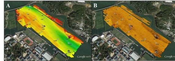
**Figure 4.** Google Earth layers of processed (A) bathymetry and (B) backscatter amplitude from data for the lower Severn River collected by the EdgeTech 6205 Swath Bathymetry and Sidescan Sonar system from the *R/V Daiber* on 02 DEC 2015.
