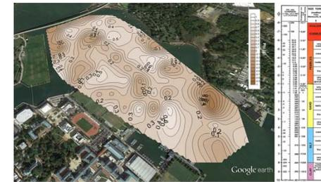
**Figure 8.** Google Earth layer of contoured  $\phi_{est}$  for the lower Severn River developed by kriging. Estimated phi values range from 1 to -1 indicative of a mean grain size between coarse and very coarse sands (<http://pubs.usgs.gov/of/2000/of00-358/text/chapter1.htm>).
