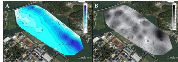
**Figure 5.** Google Earth layers for (A) bathymetry and (B) backscatter amplitude contours for the lower Severn River developed by kriging data collected by the EdgeTech 6205 Swath Bathymetry and Sidescan Sonar system from the *R/V Daiber* on 02 DEC 2015.
