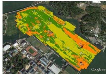
**Figure 6.** Processed backscatter amplitude in the survey area categorized and grouped into three primary return classification using ENVI software.
