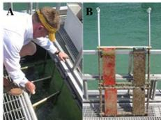
Figure 2. (A) Floor paneling being removed to lift out the mock hull plates. The deck lattice allowed ample light transmission. There are no obstructions to natural flow of water and natural processes taking place on the mock deck plates. (B) Mock hull plates removed from water to be photographed for analysis. Note the significant natural growth of algae, barnacles, bryozoans and other true biofouling agents.
