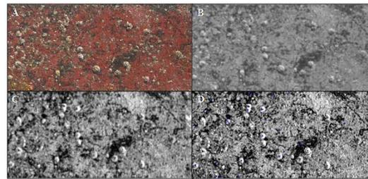
Figure 3. Series of mock hull plate images showing: (A) Hull plate picture without any contrast or color change; (B) Hull plate after an RGB split into a grey scale image with the Image-J software; (C) Hull plate with 5% contrast increase from initial grey scale image. Notice the drastic increase in distinction of barnacles from the rest of the hull plate, and; (D) Hull plate showing result of a full panel analysis trial.
