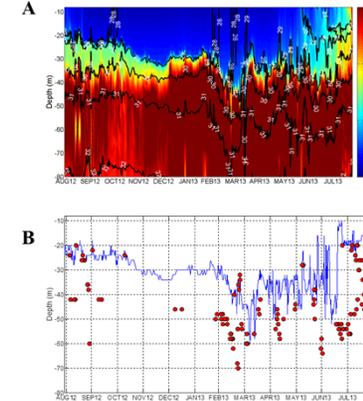
**Figure 5.** Results from ITP-64 showing: (A) A contour plot of observed temperature above the freezing point (°C) from 10 to 80 m. Salinity contours are indicated by black lines and labeled in white; and (B) A comparison of the depth of the maximum Brunt-Väisälä frequency (blue line) and the depth of the NSTM (red dots).
