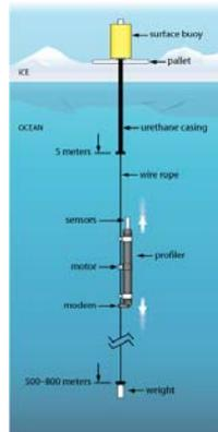
**Figure 2.** Engineering schematic of an Ice-Tethered Profiler Buoy (<http://www.whoi.edu/itp>).
