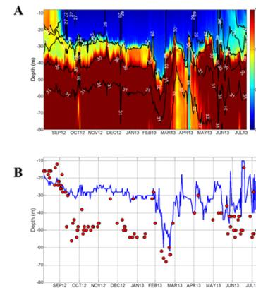
**Figure 4.** Results from ITP-62 showing: (A) A contour plot of observed temperature above the freezing point (°C) from 10 to 80 m. Salinity contours are indicated by black lines and labeled in white; and (B) A comparison of the depth of the maximum Brunt-Väisälä frequency (blue line) and the depth of the NSTM (red dots).
