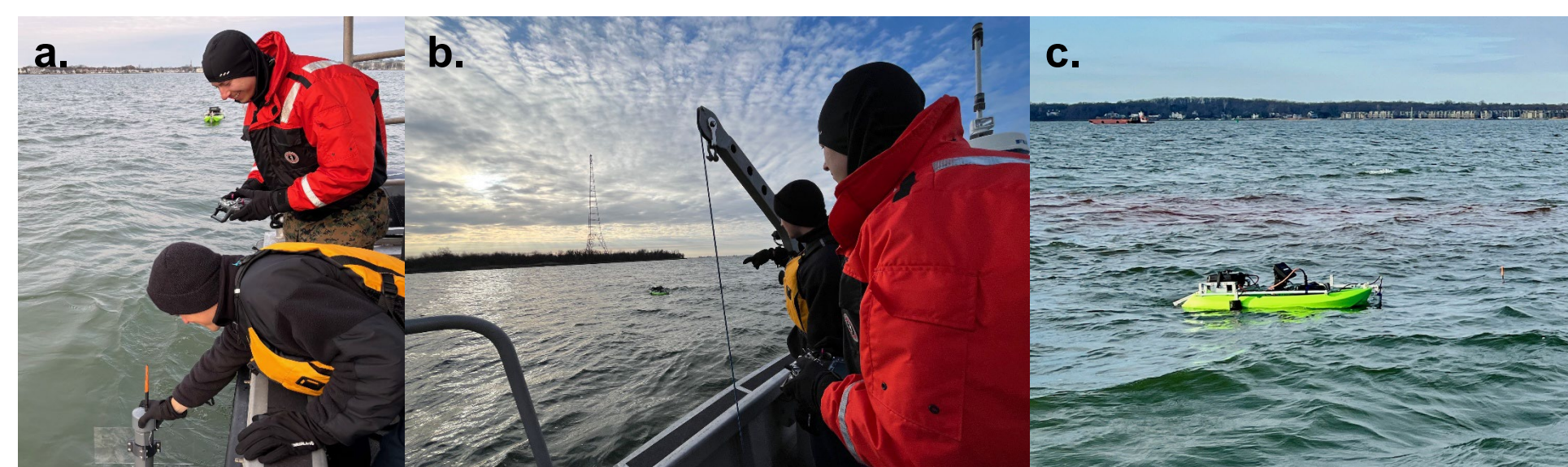
Figure 3. Midshipman 1/C Oldfield and Midshipman 1/C Guzman (a) releasing the drifter and (b) mapping the rhodamine dye plume by remote control with (c) the Coastal Kayak ASV.
