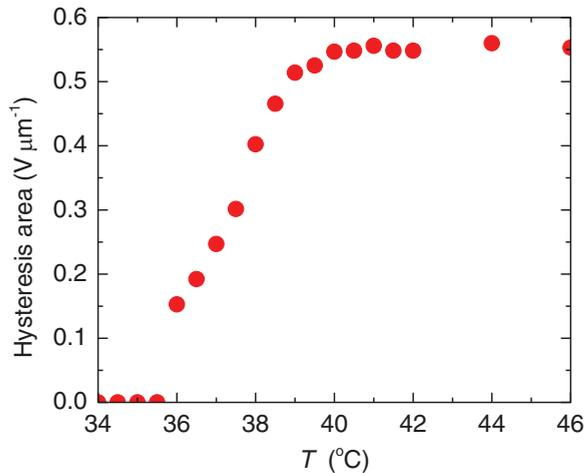
FIG. 5. (Color online) Dielectric hysteresis area for 5CB + BaTiO<sub>3</sub> (0.525 wt %) as a function of temperature. Note that  $T_{NI} = 35.5$  °C for 5CB + BaTiO<sub>3</sub> (0.525 wt %).
