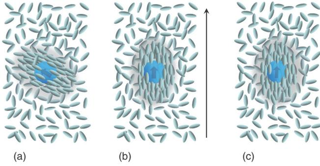
FIG. 3. (Color online) A schematic of the presence of a  $\text{BaTiO}_3$  FNP-induced pseudonematic domain in the isotropic phase. The sphere represents the FNP, the ellipsoids represent the LC molecules, and the shaded area represents the domain. (a) No electric field; (b) the electric field is turned on; (c) the electric field is turned off.
