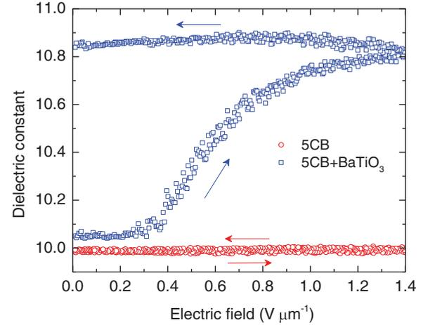
FIG. 2. (Color online) Dielectric constant as a function of the applied rms field ( $f = 1000$  Hz) in the isotropic phase ( $T = 42$  °C) for 5CB and 5CB + BaTiO<sub>3</sub> (0.525 wt %). The arrows show the field-cycle direction.
