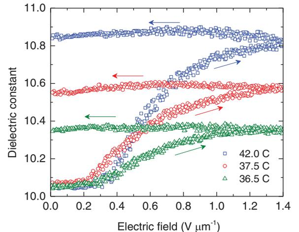
FIG. 4. (Color online) Dielectric hysteresis for  $5\text{CB} + \text{BaTiO}_3$  (0.525 wt %) at three different temperatures listed in the legend. The arrows show the field-cycle direction.
