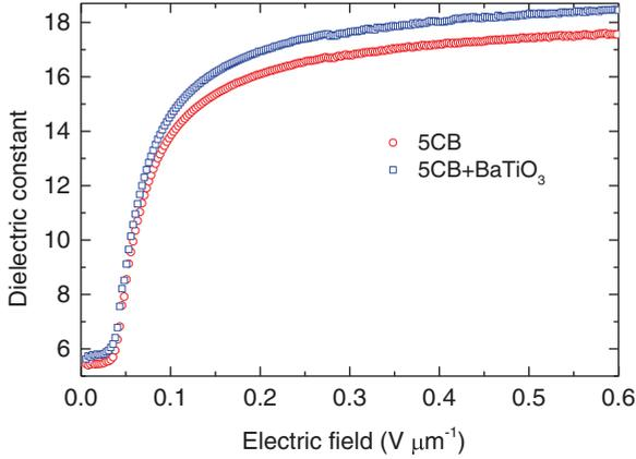
FIG. 1. (Color online) The dielectric constant as a function of applied rms field ( $f = 1000$  Hz) in the nematic phase ( $T = 25$  °C) for 5CB and 5CB + BaTiO<sub>3</sub> (0.525 wt %). This shows a typical Fréedericksz transition with a threshold field of  $0.03 \text{ V } \mu\text{m}^{-1}$ .
