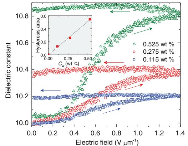
FIG. 6. (Color online) Dielectric hysteresis for 5CB + BaTiO<sub>3</sub> for three different concentrations listed in the legend. The arrows show the field-cycle direction. Inset: Hysteresis area ( $V \mu m^{-1}$ ) as a function of BaTiO<sub>3</sub> concentration in 5CB.
