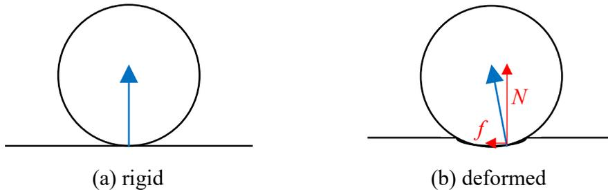
The first definition of the coefficient of rolling friction is
