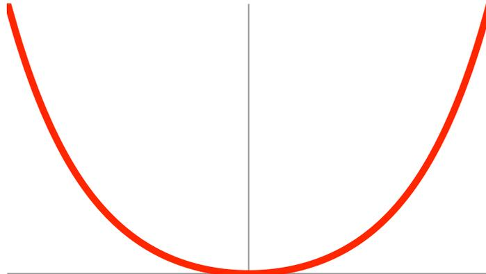
The ray comes in from the upper left and turns around vertically. Notice that both signs of the slope in Eq. (3) arise at any given value of  $z$ , except at  $z = 0$  where total internal reflection occurs.
