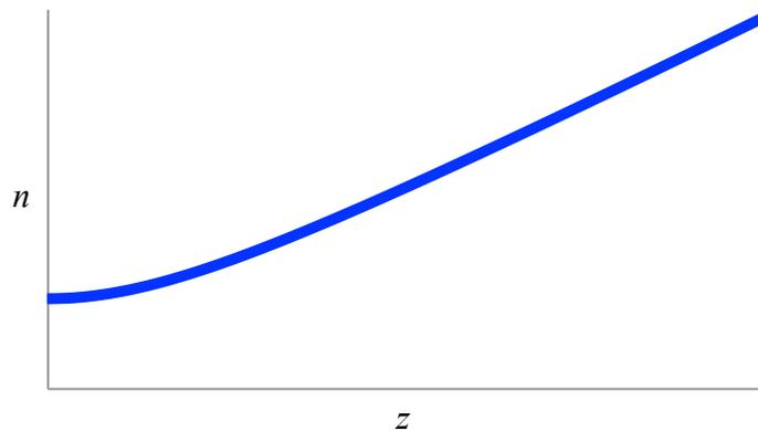
The slope approaches zero as  $z \rightarrow 0$ . That is, the index becomes constant and thus the refraction asymptotically tapers off at low altitudes. On the other hand, for large values of  $z$ , the slope
