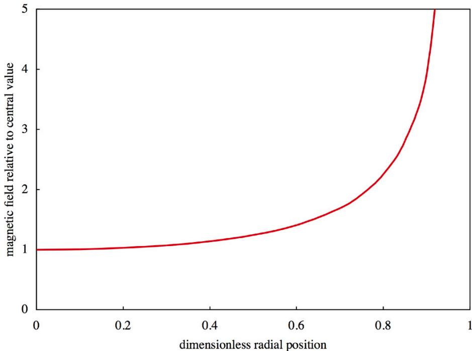
The magnetic field rises monotonically starting from the central value  $B_0$ , so using that central value to compute the inductance would lead to an underestimate. The field would diverge if  $x$  could reach  $R$ , but we prevent that by cutting it off when we hit the surface of the wire at  $x_{\max} = R - a$ .
