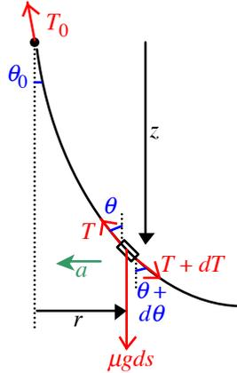
The diagram indicates the cylindrical coordinates (in black), the forces (in red), the angles of the string relative to the vertical (in blue), and the acceleration (in green) of two points along the string. At the topmost point, the tension is  $T_0$  and the angle is  $\theta_0$ . That angle cannot be zero because otherwise there would be no centripetal force on the rotating string as a whole. We will return to the two endpoints of the string later.
