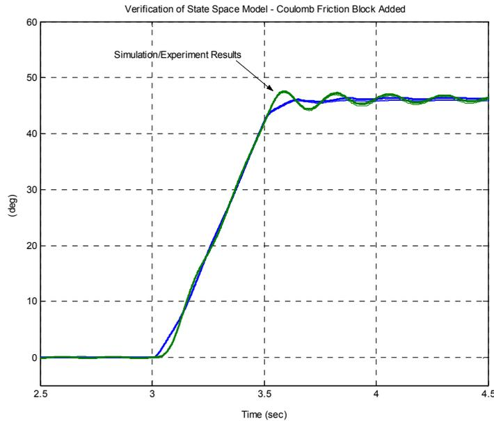
**Figure 15: Simulation and Experimental Results with Friction Block**
