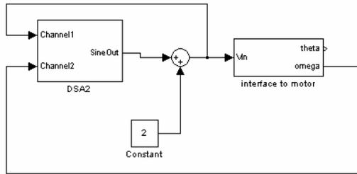
**Figure 9: Custom Bode Frequency Response Collection Diagram**
