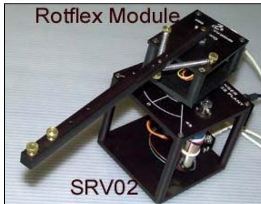
**Figure 4: Flexible Joint Robotic Arm**
