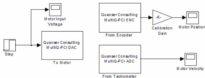
**Figure 5: SIMULINK Diagram for DC Motor Experiment**
