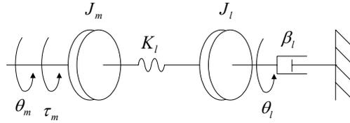
**Figure 12: DC Motor and Flexible Link Schematic**
