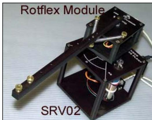
**Figure 1: Flexible Joint and DC motor.**
