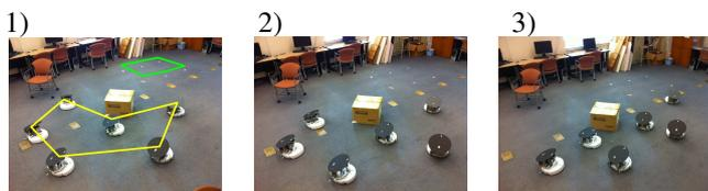
Fig. 9. Three sequential snapshots of the 6 iRobot Creates executing the motion planner presented in this paper. The first frame show the connectivity ring and the goal positions.
