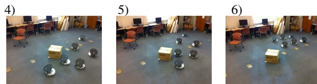
Fig. 10. Three sequential snapshots of the 6 iRobot Creates executing the motion planner presented in this paper. Frame 6 is the goal position
