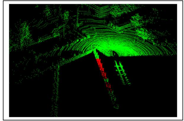
Figure 11: Using data taken from a different perspective than Figure 10, most of the dock is correctly identified (red). There are false negatives near the end where the scan is not sufficiently dense.
