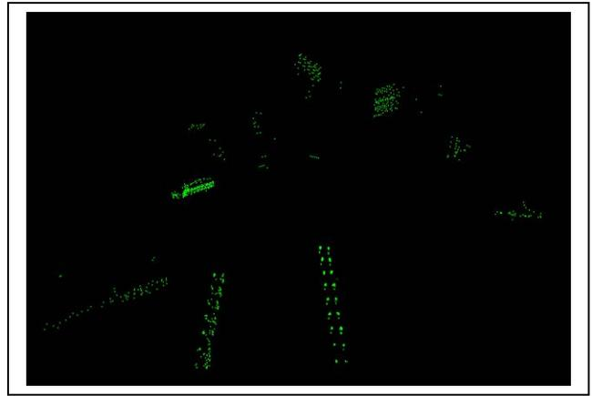
Figure 7: After removing the shore and any horizontal planar surfaces, the remaining points are grouped into clusters.
