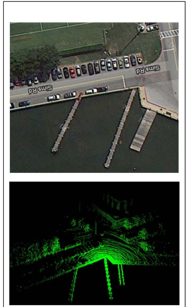
Figure 3: (top) A Google Map image of the original testing location. Note that the deck of the thick pier on the right was partially destroyed in hurricane Sandy. (bottom) A dense point cloud of the area, formed by combining three separate LiDAR scans.
