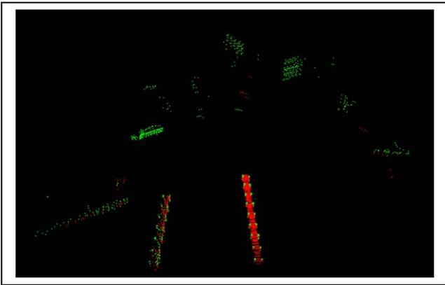
Figure 6: After the shore has been removed, RANSAC is used to identify horizontal planar surfaces (highlighted in red).
