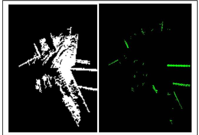
Figure 5: (left) An occupancy grid representing a bird’s eye view of the area as a binary image. (right) Morphological operations are used to eliminate most of the shore.
