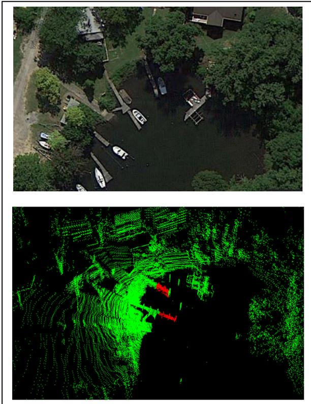
Figure 13: Point cloud data from a different test site, which includes isolated pilings, more foliage, and multiple docks – the bottom one is T-shaped. The algorithm correctly identified (red) the portions of the dock that meet our criteria.
