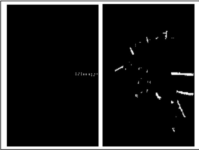
Figure 9: Using the overhead occupancy grid representation, the pilings (left) and dilated horizontal planar surfaces (right) are checked for overlap.
