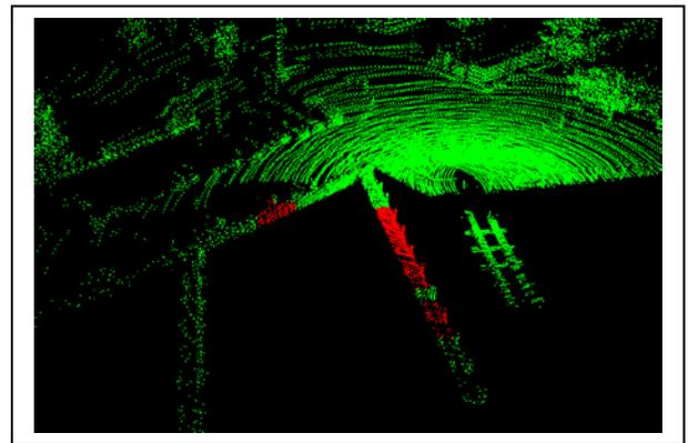
Figure 12: Using data taken from a different perspective than Figure 10, most of the dock is correctly identified (red). Note the false positive along the straight portion of the seawall longer than 4 meters.
