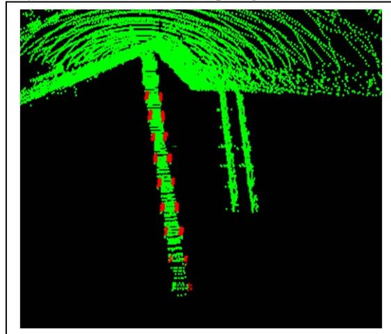
Figure 8: This close up of the point cloud shows the clusters that were identified as pilings using our Bayesian classifier (highlighted in red).
