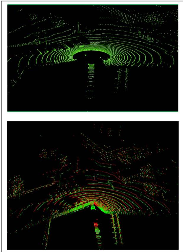
Figure 4: (top) A single LiDAR scan is not sufficiently dense to estimate the geometry of the dock. (bottom) LiDAR Scans taken from two different view-points (red and green) are registered and fused together to form a denser point cloud.
