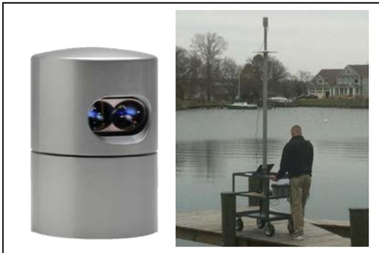
Figure 1: (left) The Velodyne HDL-32E 3-D LiDAR. (right) The LiDAR mounted on a 4 meter mast used for data collection.
