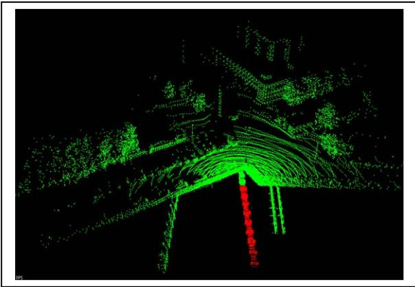
Figure 10: Using data from the scene depicted in Figure 3, the red points have been correctly identified as part of the dock. Note that the two damaged docks are not highlighted.
