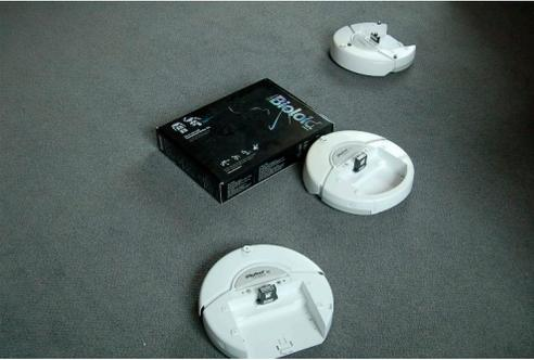
Fig. 2. Cooperative Manipulation. A group of iRobot Creates try to approach and push a box using a friction assisted grasp.
