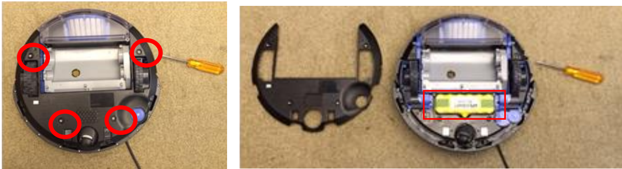
How to access battery: Remove 4 screws on (left). Lift out battery (right).
